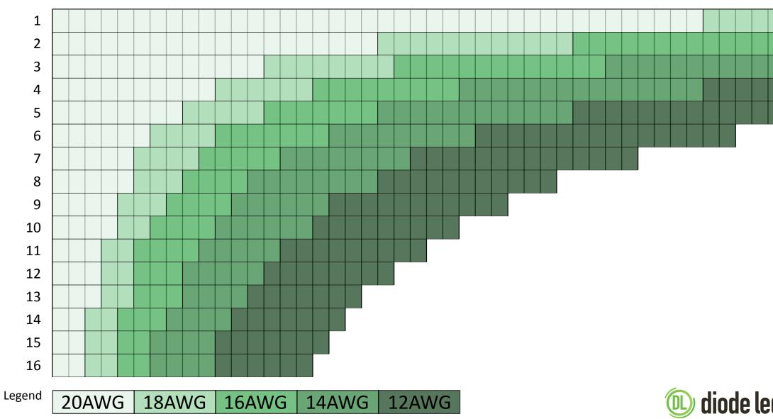
Wire lead length calculated from driver to start of LED tape light.
